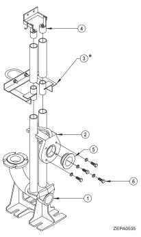
Uses 2" I.P.S. guide rails and pull cable or chain (not furnished)
