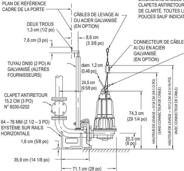
DIMENSIONS BASÉES SUR LES TAILLES DE LA NORME ANSI POUR LES CLAPETS ANTIRETOUR NéCESSAIRES, NON ILLUSTRÉS ICI POUR PLUS DE CLARTÉ. TOUTES LES DIMENSIONS SONT EN CENTIMÈTRES ET POUÇES SAUF INDICATION CONTRAIRE.
