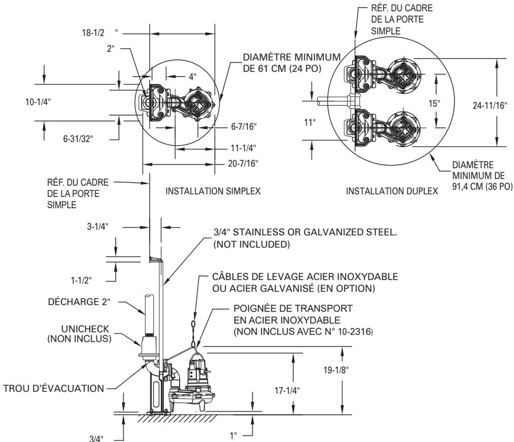
LES DIMENSIONS SONT BASÉES SUR LES TAILLES DE RACCORNS ANSI STANDARD. DES CLAPETS ANTI-RETOUR SONT NÉCESSAIRES, NON ILLUSTRÉS POUR PLUS DE CLARTÉ.
