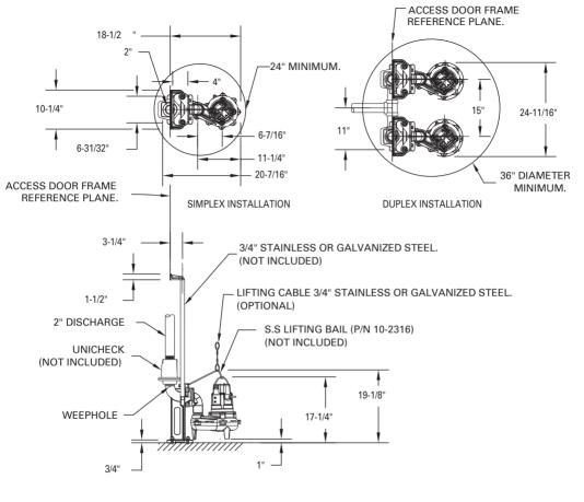
DIMENSIONS ARE BASED ON STANDARD ANSI FITTING SIZES. CHECK VALVES ARE REQUIRED, NOT SHOWN FOR CLARITY. ALL DIMENSIONS IN INCHES UNLESS OTHERWISE NOTED. MINIMUM SIZE IS FOR PHYSICAL FIT ONLY, PUMP VOLUME/OPERATION MAY REQUIRE LARGER BASIN.
