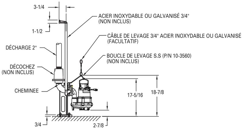
LES DIMENSIONS SONT BASÉES SUR LES TAILLES DE RACCORDS ANSI STANDARD. VÉRIFIER QUE LES VALVES SONT NÉCESSAIRES, NON ILLUSTRÉ POUR PLUS DE CLARTÉ. TOUTES LES DIMENSIONS EN POUCES SAUF INDICATION CONTRAIRE. LA TAILLE MINIMALE EST UNIQUEMENT POUR L'AJUSTEMENT PHYSIQUE, LE VOLUME/LE FONCTIONNEMENT DE LA POMPE PEUT NÉCESSAIREMENT UN BASSIN PLUS GRAND.
