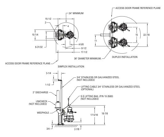
DIMENSIONS ARE BASED ON STANDARD ANSI FITTING SIZES. CHECK ARE VALVES REQUIRED, NOT SHOWN FOR CLARITY. ALL DIMENSIONSIN INCHES UNLESS OTHERWISE NOTED. MINIMUM SIZE IS FOR PHYSICAL FIT ONLY, PUMP VOLUME/OPERATION MAY REQUIRE LARGER BASIN.
