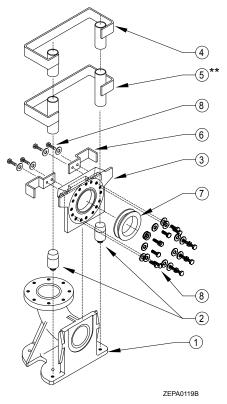
\* NOTE: Discharge Elbow 006574 Revision A & B will have Stainless Steel Lower Guides, and Revision C will have Cast Iron Lower Guides. \*\* Optional: order P/N 6039-0014 for pit depths greater than 15 ft. Uses 2" I.P.S. guide rails and pull cable or chain (not furnished)
