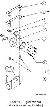
\* Not replaceable - order complete discharge elbow.
