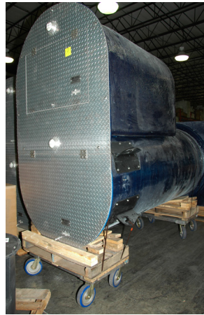
Duplex wet well valve box
