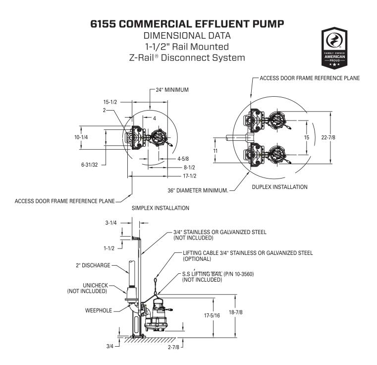
DIMENSIONS ARE BASED ON STANDARD ANSI FITTING SIZES. CHECK ARE VALVES REQUIRED, NOT SHOWN FOR CLARITY. ALL DIMENSIONSIN INCHES UNLESS OTHERWISE NOTED. MINIMUM SIZE IS FOR PHYSICAL FIT ONLY, PUMP VOLUME/OPERATION MAY REQUIRE LARGER BASIN. BASIN DEPTHS GREATER THAN 12' DEEP WILL REQUIRE A #39-0139 INTER MEDIATE STABILIZER BRACKET.
