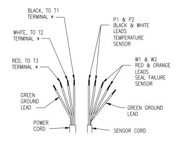
\* TERMINALS T1, T2 AND T3 IDENTIFY MAGNETIC STARTER TERMINAL CONNECTIONS.
