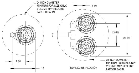
DIMENSIONS BASED ON STD. ANSI FITTING SIZES CHECK VALVES REQUIRED, NOT SHOWN FOR CLARITY ALL DIMENSIONS IN INCHES UNLESS OTHERWISE NOTED
