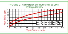
Once the peak flow rate of the drain line into the sewage lift station has been determined, pump capacity should be equal to that flow. If it is always critical that fixtures be kept in operation, a duplex pump station should be specified in lieu of a simplex station. In case of a pump failure, the other pump could carry the load while the failed pump is being repaired.
